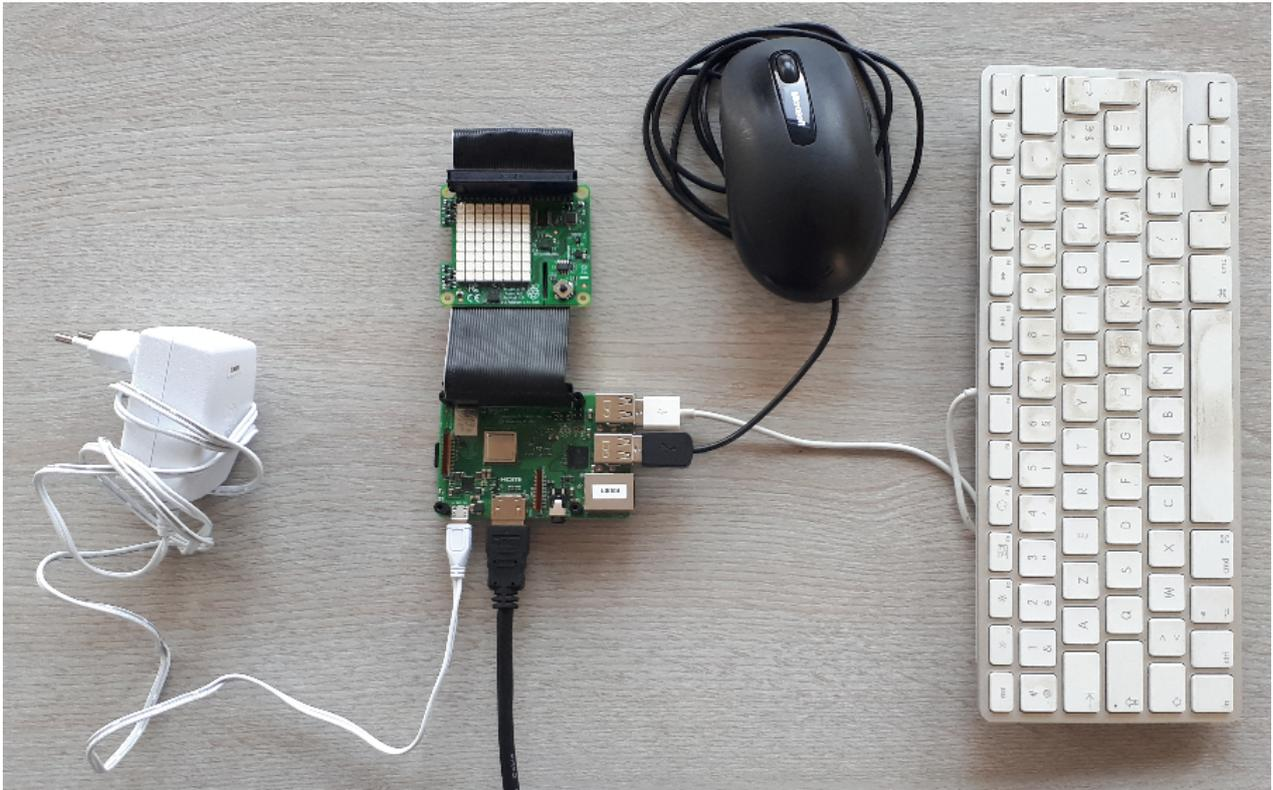
*Figure 1: Connections of the Raspberry board*
